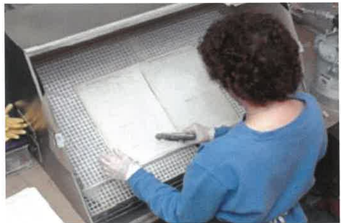
Weak, brittle, badly torn, and fragmented maps are mounted on Japanese tissue, primarily Kozo or Zangetsu. Mending mildly torn maps is performed using either Japanese tissue and ethyl cellulose paste or
